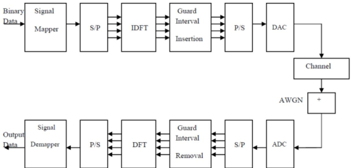
Figure 2: The basic block diagram of an OFDM system in AWGN channel
