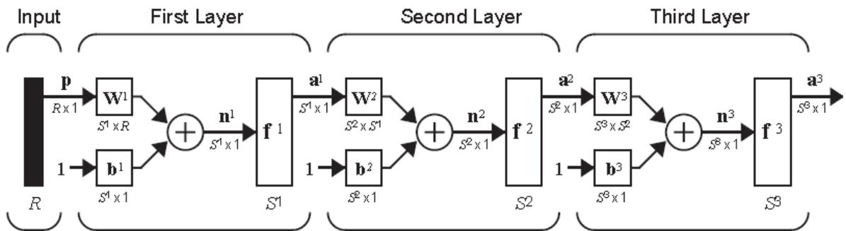
Figure 13: A Multi-Layer Feed Forward Network with 3 hidden layers
