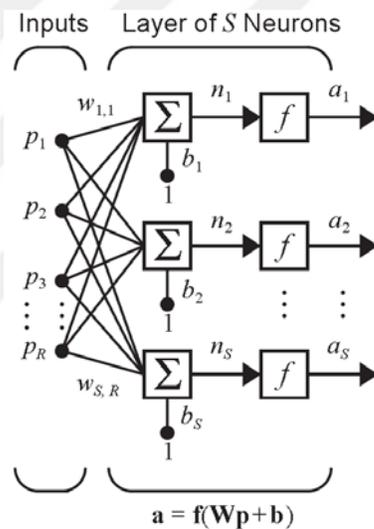
Figure 12: Structure of a simple Feed Forward ANN with  $R$  inputs, and  $S$  number of neurons in hidden layer
