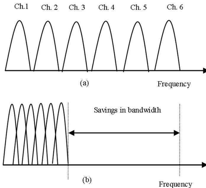
Figure 1: (a) Multiple Carriers in FDM, (b) Multiple Orthogonal Carriers in OFDM
