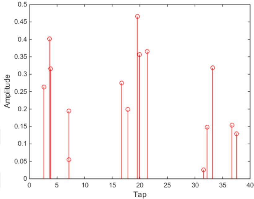
Figure 4: Sparse Multipath Channel
