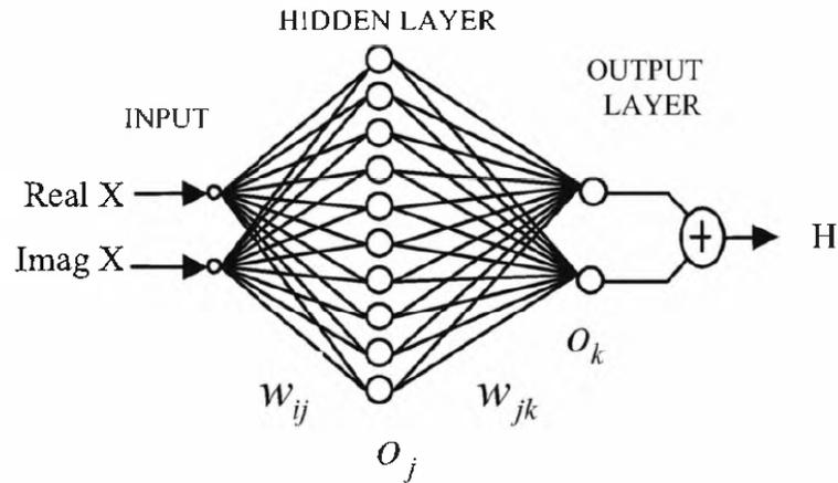
Figure 14: MLP-ANN model used with separate Real and Imaginary Inputs
