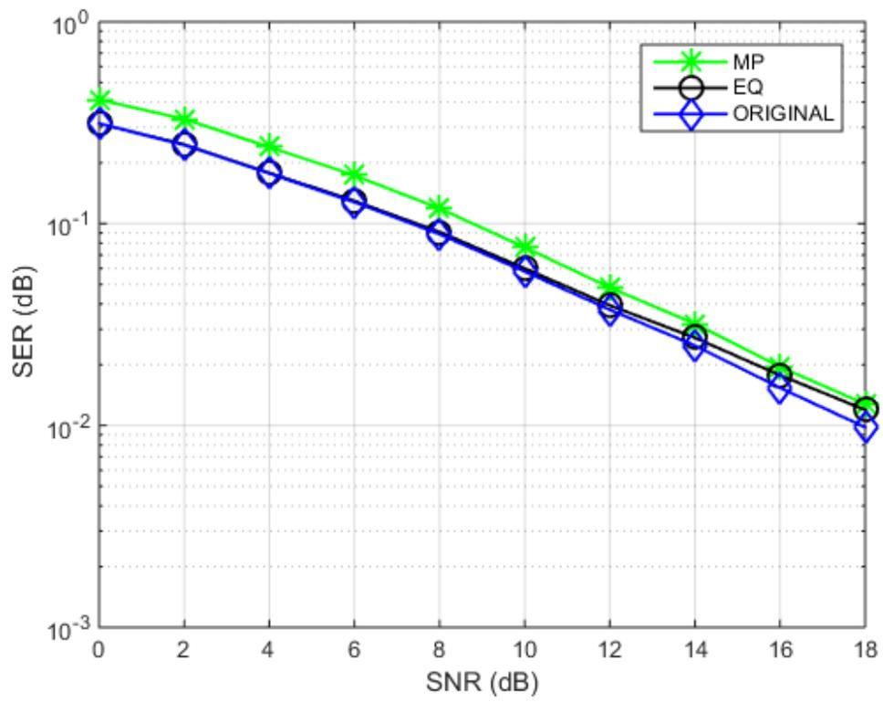
Figure 10: Performance comparison for MP estimate, original and equalized channel ( $\rho = 20, \gamma = 4$ )
