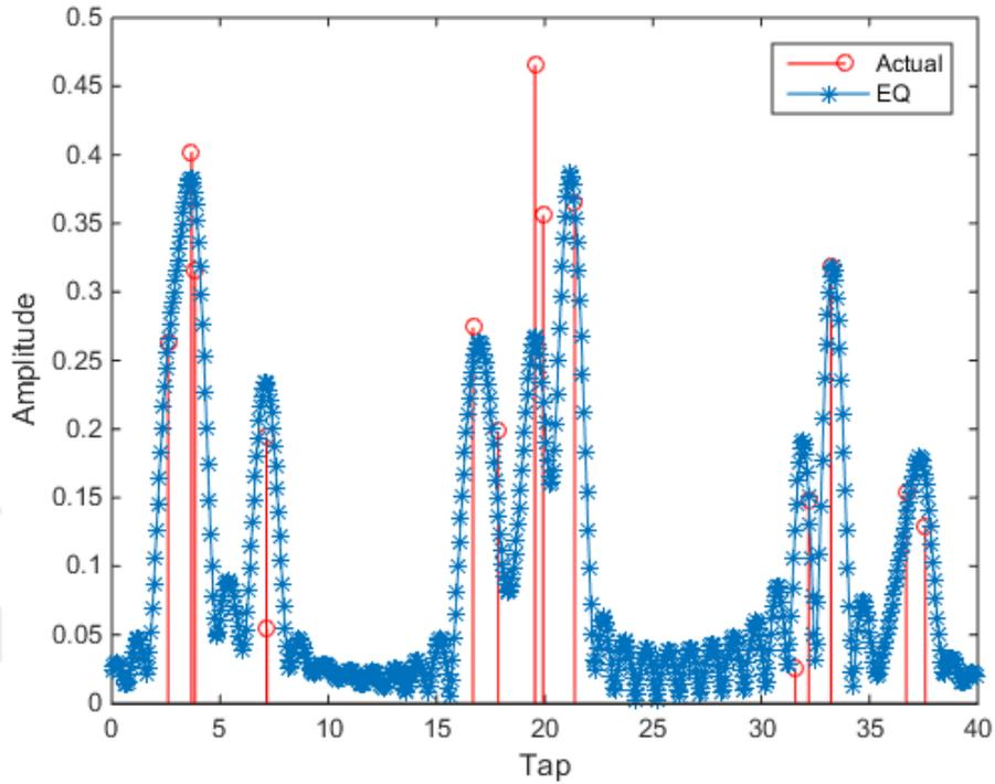
Figure 5: Time-Domain representation of the Sparse-multipath channel and its equivalent channel ( $\rho = 16$ )
