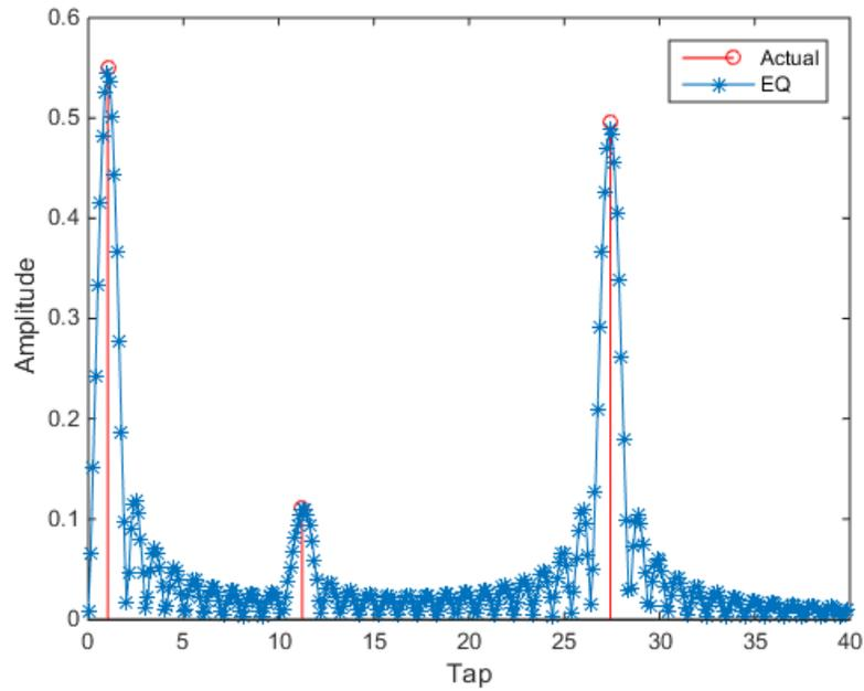
Figure 6: Time-Domain representation of the Sparse-multipath channel and its DT equivalent channel ( $\rho=8$ )
